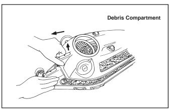
Figure 3. Remove Debris compartment
